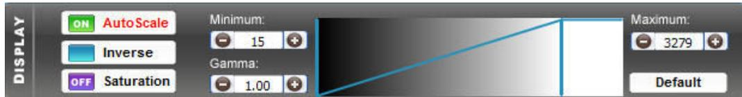
The acquired images are for instance 12-bit ones, ranging from 0 up to 4 095 grey levels. Windows® can only display 8 bit images (256 grey levels).
