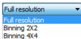
The Quantum ST4 system offers exquisite resolution of more than 1.4 million pixels to maximize quantifiable data. The system can be used at either its full resolution or with binning.
