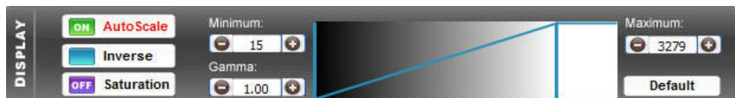
The acquired images are for instance 12-bit ones, ranging from 0 up to 4 095 grey levels. Windows® can only display 8 bit images (256 grey levels).
