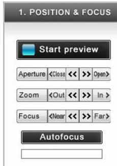
The zoom control dialog box is displayed each time the acquisition menu is active. It helps you to adjust the 3 settings of the zoom lens:
