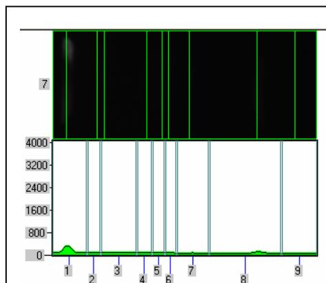
Display of the profile from 0 to the maximum dynamic (i.e.: 255 for a 8-bit image and 16 384 for a 14-bit image).
