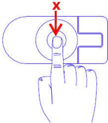
To open the door: Push the button "X" with the finger and lift the handle.
