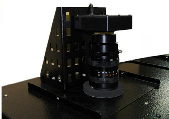
**Illustration 4:** the camera/optics installed on the top of the darkroom (front side)
