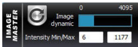
The image dynamic refers to the range of grey levels in between the minimum and the maximum pixel intensities obtained in an image.
