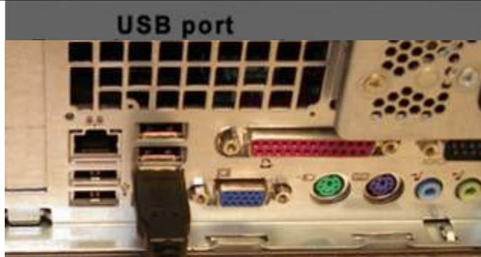
⇒ Connect the cable coming from the USB camera to the computer USB port.
