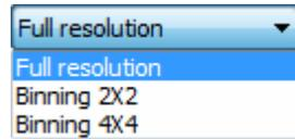
The binning technique combines the charge from adjacent pixels so that the total charge can be read-out as a single pixel.
