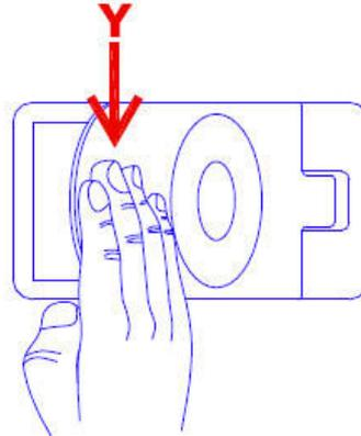
To close the door: Close the door and block it by pushing the part "Y".
