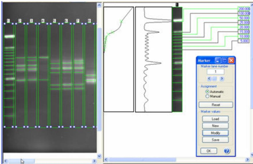
Note: The migration curve allows to check the detection of value application errors, distortion errors, bad separation between the bands, or the quality of the standard itself.
