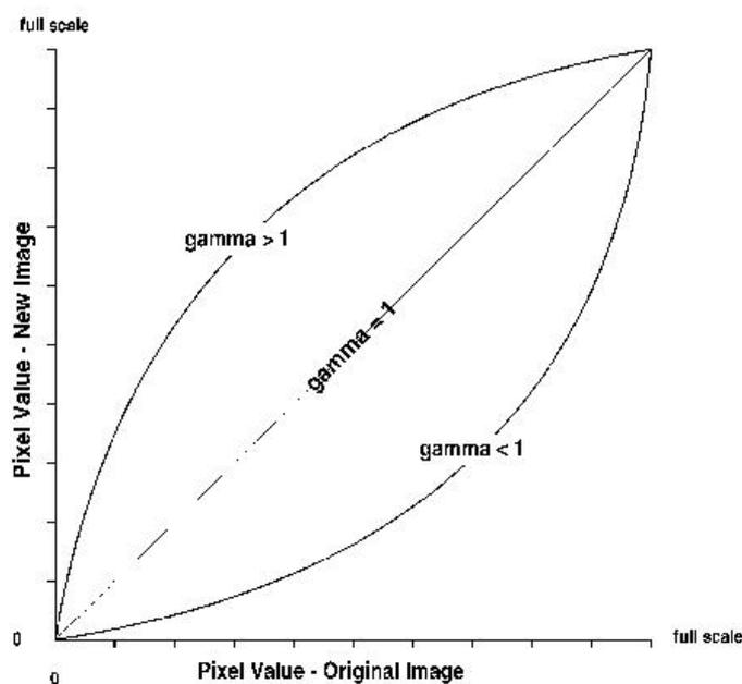
The above graph demonstrates the basic principles of gamma adjustment:
