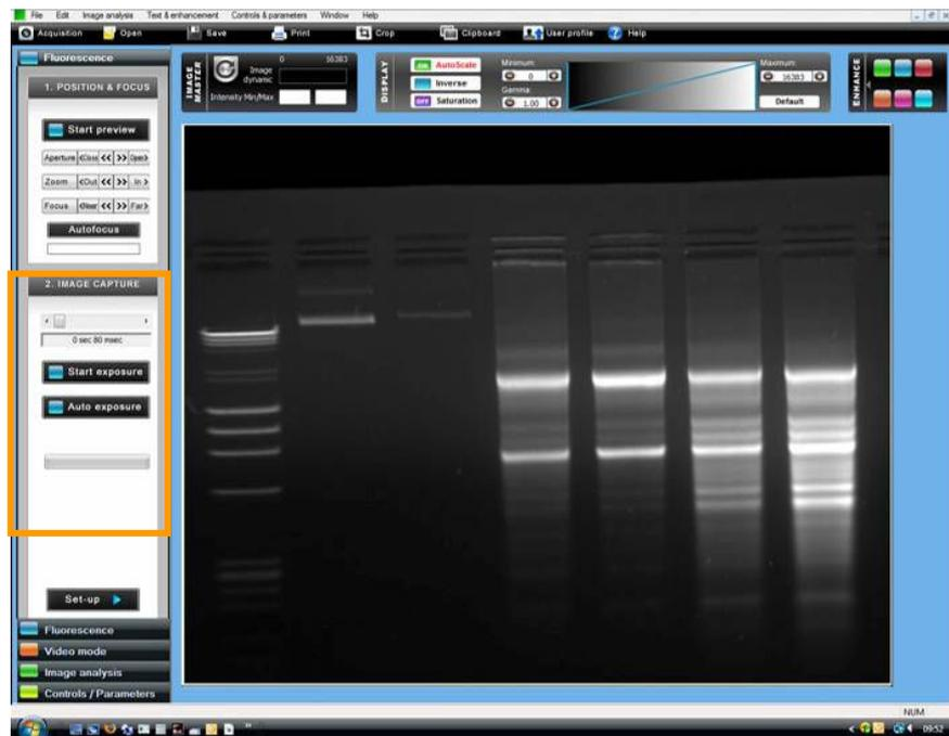
To adjust the exposure time, adjust the scroll bar position:
