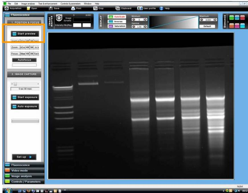
Note: A live image means the image displayed is refreshed every 1/20th of a second. This short exposure time (or frame) is adequate for a variety of white light samples including protein gels and autoradiography. A live image, however, is not sufficient for most samples, which are visualised and photographed over a relatively dim UV light source. A feature called integration compensates the low light situation by allowing the CCD camera to obtain a timed exposure.
