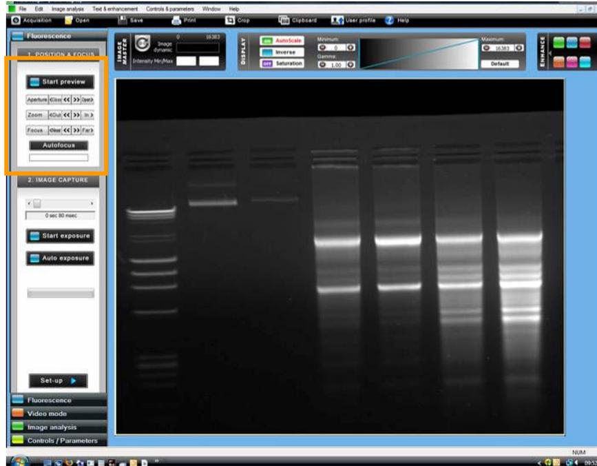
All cameras require a focus point adjustment. In order to proceed, you have to zoom to the maximum on a straight forward image (a printed paper, a business card ...). Then, focus till you obtain a very sharp image on the screen. This procedure can be done with epi-illumination light and a printed paper. The focus point adjustment varies with the focal distance.
