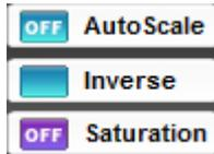
A saturated image is inappropriate for image quantification with image analysis software. The saturation option allows you to visualise in red, pixels that have the maximum grey level (4095) in order to avoid to flatten the peaks.
