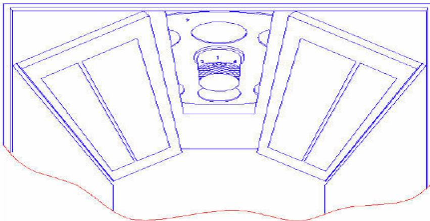
The first position is designed for the F590 filter for ethidium bromide application, at UV transilluminator level (if any).
