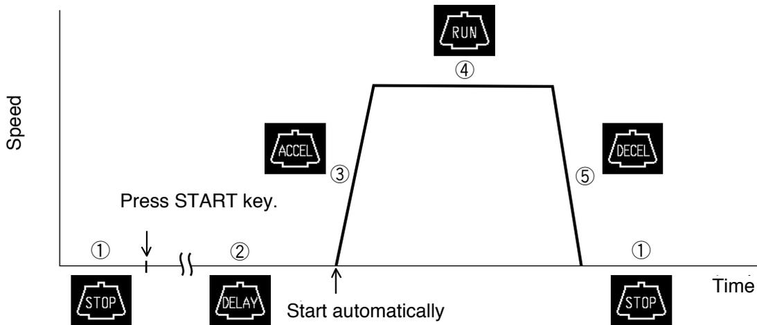
Fig. 3-3-6 Operating mode (RTC)
