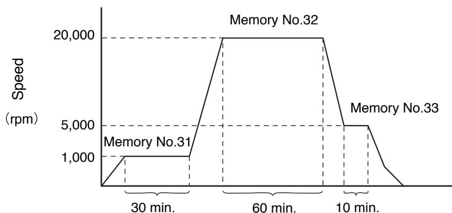
Fig. 3-3-2 Details of an example step-mode operation
