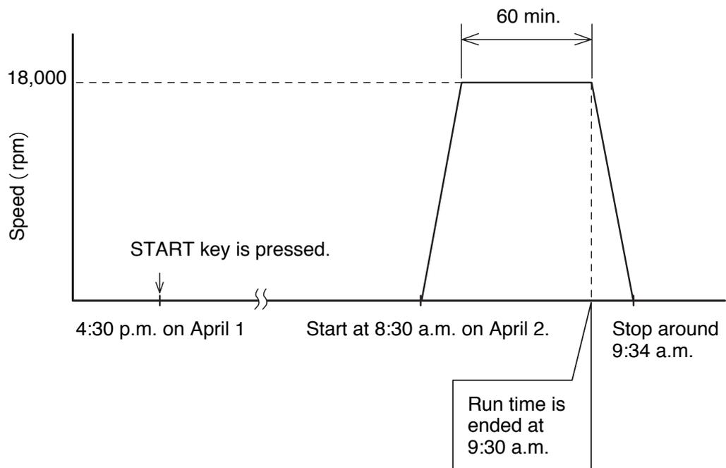
Fig. 3-3-5 Example of RTC operation
