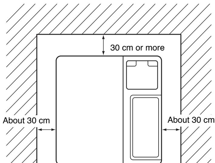
Fig. 6-1 Clearances for centrifuge
